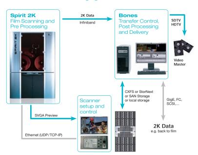
The combination of the Spirit 2K film scanner and Bones open post-production system scans film in 2K resolution, which is then stored on disk using the Bones Transfer and Bones Mover applications. In the diagram below, the Spirit 2K system is set up with a graphical control panel (GCP), which is part of the basic scanner unit. The 2K data is then post processed via the Bones system and formatted into the desired output format: data, SD, or HD.
